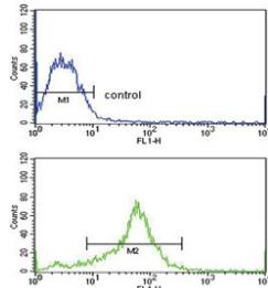
Flow cytometry testing of human MCF7 cells with TIMP3 antibody; Blue=isotype control, Green= TIMP3 antibody.
