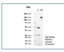
SDS-PAGE analysis of purified, BSA-free Syndecan-1 antibody (clone SDC1/7178) as confirmation of integrity and purity.
