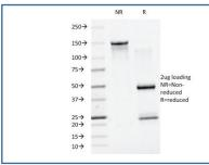
SDS-PAGE analysis of purified, BSA-free SUMO1 antibody (clone SM1/495) as confirmation of integrity and purity.
