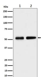
Western blot analysis of Septin 8 expression in (1) human HeLa cell lysate; (2) mouse NIH 3T3 cell lysate using SEPTIN8 antibody. Predicted molecular weight ~56 kDa.
