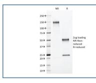
SDS-PAGE analysis of purified, BSA-free S100B antibody (clone 4C4.9) as confirmation of integrity and purity.
