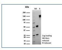
SDS-PAGE analysis of purified, BSA-free S100A4 antibody (clone S100A4/6799) as confirmation of integrity and purity.
