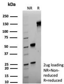
SDS-PAGE analysis of purified, BSA-free S100A4 antibody (clone S100A4/6799) as confirmation of integrity and purity.
