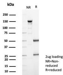
SDS-PAGE analysis of purified, BSA-free S100 calcium-binding protein A13 antibody (clone S100A13/7482) as confirmation of integrity and purity.
