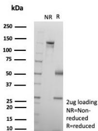
SDS-PAGE analysis of purified, BSA-free recombinant SMAD4 antibody (clone SMAD4/7906R) as confirmation of integrity and purity.
