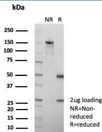
SDS-PAGE analysis of purified, BSA-free recombinant ROR gamma antibody (clone RORC/8278R) as confirmation of integrity and purity.
