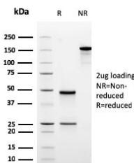
SDS-PAGE analysis of purified, BSA-free recombinant ODC1 antibody (clone rODC1/485) as confirmation of integrity and purity.
