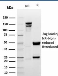
SDS-PAGE analysis of purified, BSA-free recombinant Myogenin antibody (clone MYOG/6298R) as confirmation of integrity and purity.
