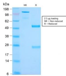
SDS-PAGE analysis of purified, BSA-free recombinant MUC2 antibody (clone MLP/2970R) as confirmation of integrity and purity.
