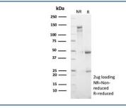
SDS-PAGE analysis of purified, BSA-free recombinant MKI67 antibody (clone rMKI67/9616) as confirmation of integrity and purity.
