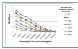
ELISA Titration: the plate was coated with different amounts of human IgA2. A serial dilution of recombinant Human IgA2 antibody was used as the primary and an alkaline phosphatase conjugated anti-rabbit IgG as the secondary.
