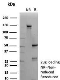
SDS-PAGE analysis of purified, BSA-free recombinant CNN1 antibody (clone rCNN1/9164) as confirmation of integrity and purity.
