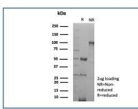
SDS-PAGE analysis of purified, BSA-free recombinant CKB antibody (clone rCKBB/8839) as confirmation of integrity and purity.
