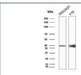
Western blot testing of human HEK293 and Y79 cell lysate with recombinant CKB antibody. Predicted molecular weight ~43 kDa.
