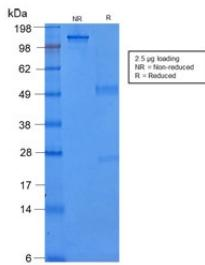
SDS-PAGE analysis of purified, BSA-free recombinant CK8 antibody (clone rB22.1) as confirmation of integrity and purity.
