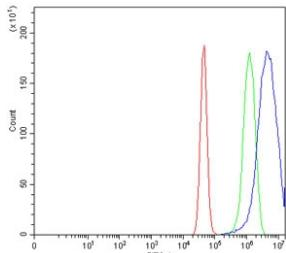
Flow cytometry testing of human U-87 MG cells with Ran GTPase-activating protein 1 antibody at 1ug/million cells (blocked with goat sera); Red=cells alone, Green=isotype control, Blue= Ran GTPase-activating protein 1 antibody.
