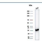
Western blot testing of human Raji cell lysate with Proliferating Cell Nuclear Antigen antibody (clone PCNA/8303R). Predicted molecular weight ~29 kDa, routinely observed at 29~36 kDa.
