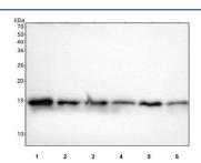
Western blot testing of 1) human HepG2, 2) human HeLa, 3) rat liver, 4) rat brain, 5) mouse liver and 6) mouse brain tissue lysate with PIN4 antibody. Predicted molecular weight ~14 kDa.
