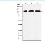
Western blot testing of 1) human K562, 2) mouse RAW264 and 3) rat kidney lysate with PIK3CD antibody. Expected molecular weight: 110-120 kDa.
