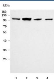
Western blot testing of human 1) U-87 MG, 2) MCF7, 3) HeLa and 4) SiHa cell lysate with PHTF1 antibody. Predicted molecular weight ~87 kDa but may be observed at higher molecular weights due to glycosylation.
