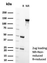
SDS-PAGE analysis of purified, BSA-free Nucleolin antibody (clone NCL/7339) as confirmation of integrity and purity.
