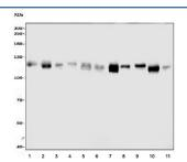
Western blot testing of human 1) HEK293, 2) K562, 3) U-2 OS, 4) Jurkat, 5) HeLa, 6) ThP-1, 7) Caco-2, 8) rat brain, 9) rat PC-12, 10) mouse lung and 11) mouse brain tissue lysate with NOTCH1 antibody. Expected molecular weight: ~ 270 kDa (full length), ~ 120 kDa (transmembrane fragment).
