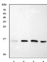
Western blot testing of 1) human U937, 2) rat lung, 3) mouse lung and 4) mouse spleen tissue lysate with Lysozyme C antibody. Expected molecular weight ~17 kDa.
