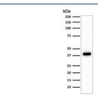
Western blot testing of HCT116 cell lysate with Cytokerain 18 antibody (clone C-04). Expected molecular weight: 46-50 kDa.
