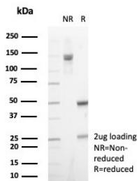
SDS-PAGE analysis of purified, BSA-free HCG-alpha antibody (clone rHCGa/6975) as confirmation of integrity and purity.
