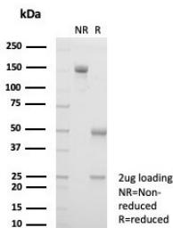
SDS-PAGE analysis of purified, BSA-free Haptoglobin antibody (clone HP/3838) as confirmation of integrity and purity.
