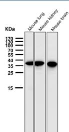
All lanes use the GGH antibody at 1:1000 dilution for 1 hour at room temperature. Expected molecular weight ~36 kDa but additional bands may be observed due to glycosylation.
