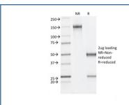
SDS-PAGE analysis of purified, BSA-free FBN1 antibody (clone FBN1/2191) as confirmation of integrity and purity.
