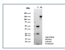
SDS-PAGE analysis of purified, BSA-free FABP1 antibody (clone FABP1/4519) as confirmation of integrity and purity.
