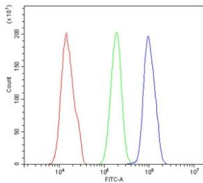
Flow cytometry testing of human HeLa cells with EYA4 antibody at 1ug/million cells (blocked with goat sera); Red=cells alone, Green=isotype control, Blue= EYA4 antibody.
