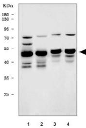
Western blot testing of 1) human HepG2, 2) human RT4, 3) rat brain and 4) mouse brain tissue lysate with EAP2 antibody. Expected molecular weight: 41-51 kDa.
