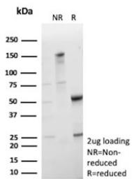
SDS-PAGE analysis of purified, BSA-free CLPS antibody (clone CLPS/9902) as confirmation of integrity and purity.
