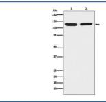
Western blot testing of 1) human HeLa and 2) mouse RAW 264 cell lysate with Chromogranin B antibody. Predicted molecular weight ~78 kDa but may be observed at up to ~120 kDa.
