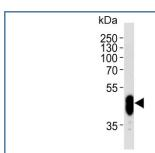
Western blot testing of human brain lysate with CDK14 antibody. Predicted molecular weight ~53 kDa.
