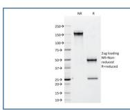
SDS-PAGE analysis of purified, BSA-free CD79b antibody (clone IGB/1842) as confirmation of integrity and purity.
