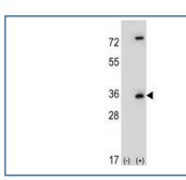
Western blot analysis of Caspase-3 antibody and 293 cell lysate (2 ug/lane) either nontransfected (Lane 1) or transiently transfected (2) with the CASP3 gene.
