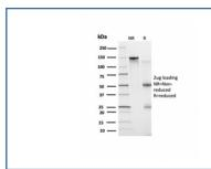
SDS-PAGE analysis of purified, BSA-free Bcl6 antibody (clone PCRP-BCL6-1D3) as confirmation of integrity and purity.
