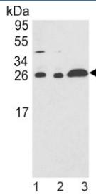
Western blot testing of human 1) A375, 2) HL60 and 3) Ramos cell lysate with ARHGDIA antibody. Expected molecular weight: 23-29 kDa.
