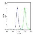
Flow cytometry testing of fixed and permeabilized human U-87 MG cells with APLP1 antibody; Blue=isotype control, Green= APLP1 antibody.
