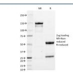
SDS-PAGE analysis of purified, BSA-free IgA antibody (clone IA761) as confirmation of integrity and purity.
