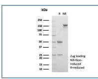
SDS-PAGE analysis of purified, BSA-free AMBP antibody (clone AMBP/4533) as confirmation of integrity and purity.
