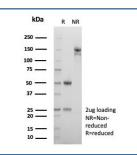
SDS-PAGE analysis of purified, BSA-free A2M antibody (clone A2M/4847) as confirmation of integrity and purity.
