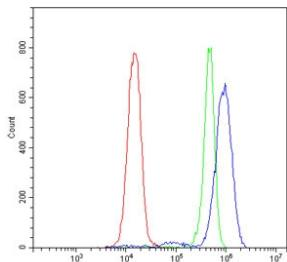
Flow cytometry testing of human Jurkat cells with STAT5b antibody at 1ug/million cells (blocked with goat sera); Red=cells alone, Green=isotype control, Blue= STAT5b antibody.
