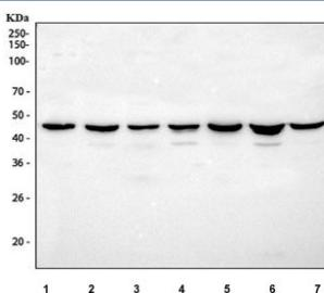
Western blot testing of 1) human Jurkat, 2) human HEL, 3) human RT4, 4) rat testis, 5) rat PC-12, 6) mouse testis and 7) mouse RAW264.7 cell lysate with APOBEC3G antibody at 0.5ug/ml. Predicted molecular weight: ~46 kDa.
